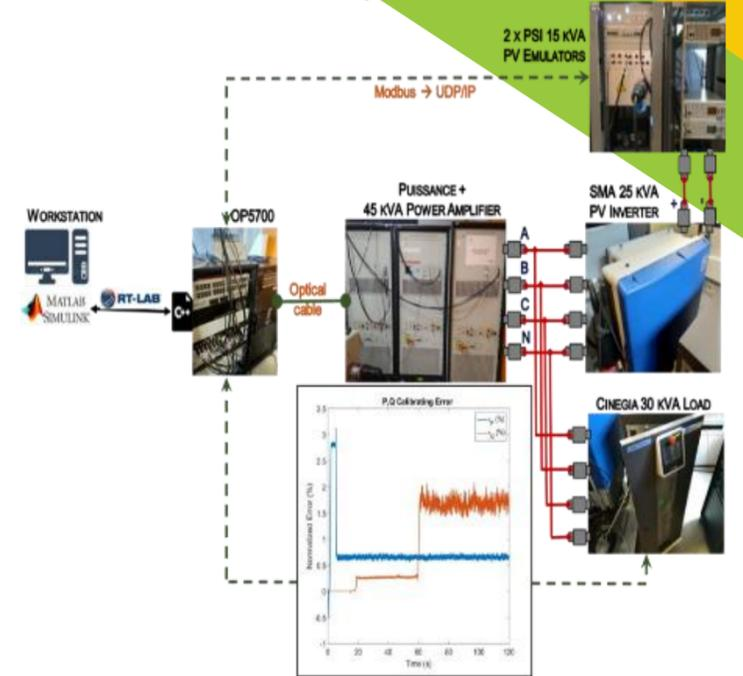
Fig1 : Voltage and frequency control in isolated µgrid by real time simulation (HIL)
